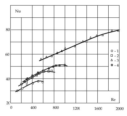
Fig.1. The dependence of the Nusselt number on the Reynolds number: Gravel particles with an average diameter  $d_{av}$ , mm: 1-1,98; 4-3,04; Glass particles with an average diameter  $d_{av}$ , mm: 2-2,37; 3-4,47.
